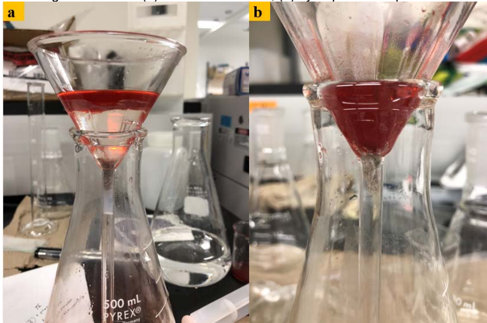
Figure 2: Application in oil-water separation: (a) initial immiscible oil-water; (b) separation after 15 min
