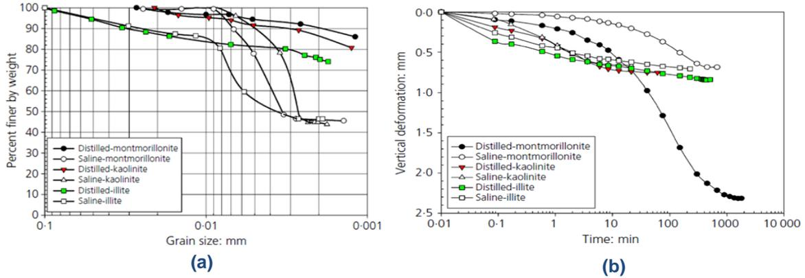
**Figure 5: (a)** Particle size distributions of different soil samples treated with NaCl solution **(b)** Changes in vertical deformation of treated and untreated soil samples with time (Tiwari and Ajmera, 2014).
