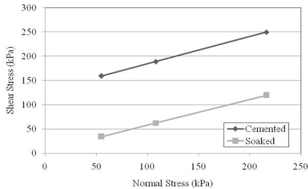
**Figure 6:** Soaking effect on shear strength of saline soil (Moayed et al., 2011).
