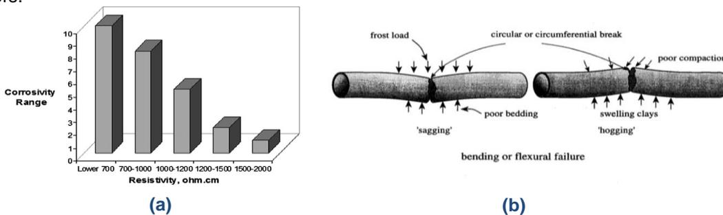
**Figure 8: (a)** The increase of soil resistivity with the increase of salt concentrations in soil leads to increase the potential of soil corrosion (Ismail and El-shamy 2009); **(b)** The failure of water mains pipelines due to poor bedding support and clay swelling (Rajani et al. 1996).
