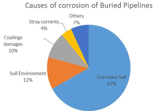
**Figure 9:** Factors affecting the failure of metal buried pipeline due to corrosion (Romer et al. 2004).
