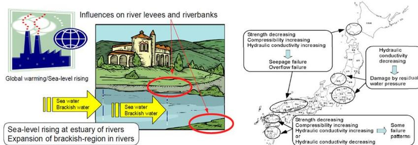
**Figure 1:** Damage patterns of river bank and levees due to sea-level rising in Japan (Komine, 2007a; Komine, 2007b).
