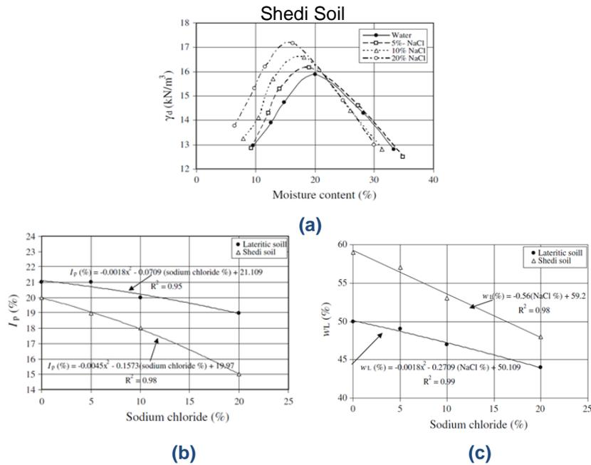
**Figure 4:** Effect of NaCl on: (a) compaction characteristics of Shedi Soil; (b) liquid limit; and (c) plastic limit of Lateritic and Shedi Soils (Nayak et al., 2010).
