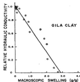
**Figure 2.** Macroscopic swelling for clayey soil versus relative hydraulic conductivity (McNeal et al., 1966).
