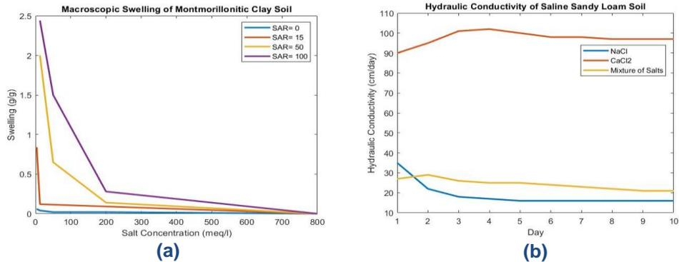
**Figure 3: (a)** Macroscopic Swelling potential of Gila clay soil under different sodium content. (Note: SAR= Sodium Adsorption Ratio =  $\left(\frac{Na^+}{\sqrt{\frac{1}{2}(Ca^{2+}+Mg^{2+})}}\right)$ ). **(b)** Hydraulic conductivity of saline sandy loam soil over time during leaching of salt solutions (e.g. NaCl and CaCl<sub>2</sub>) and mixture of salts.
