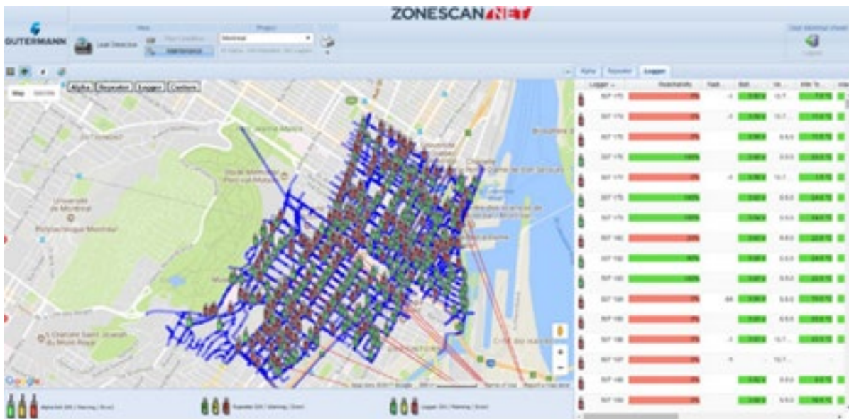
Figure 3: Noise loggers leak detection interface – City of Montreal
