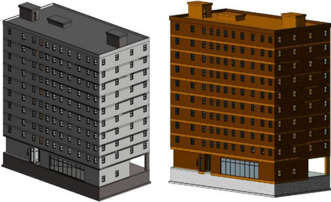
Figure 2 Two 10-storey buildings: concrete and steel frame (left) Full CLT (right)
