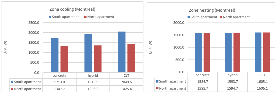
Figure 6. Peak loads of buildings in Montreal
