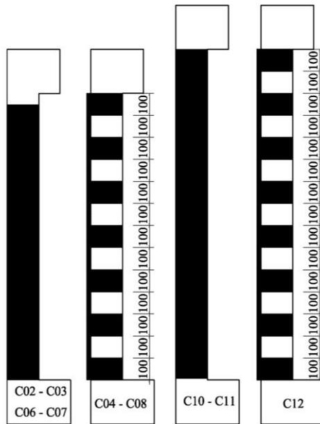
Figure 2: Strengthening Schemes of Wrapped Specimens
