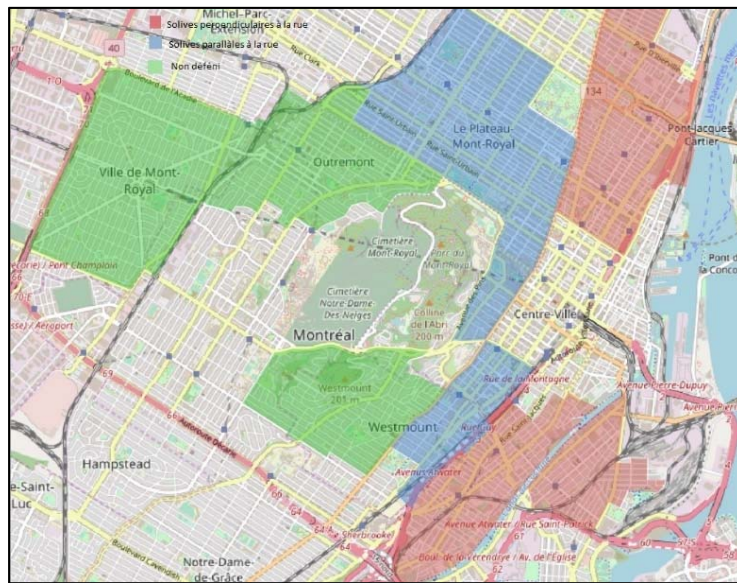
Figure 1: Location of URM-B1 buildings (Internal wood framing supported by URM firewalls (Blue), by façade and rear URM walls (Red) or unknown (Green)).
