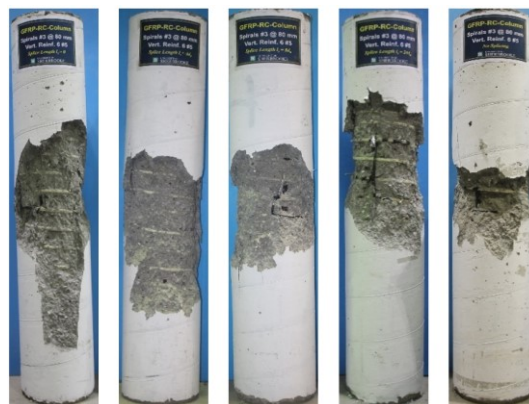
G5-L0-80 G5-L4-80 G5-L8-80 G5-L24-80 G5-LC80 Figure 9. Overview of the column specimens after failure.
