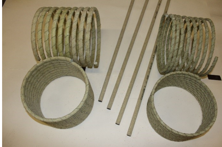
Figure 2. Sand-coated GFRP spirals and straight reinforcement.
