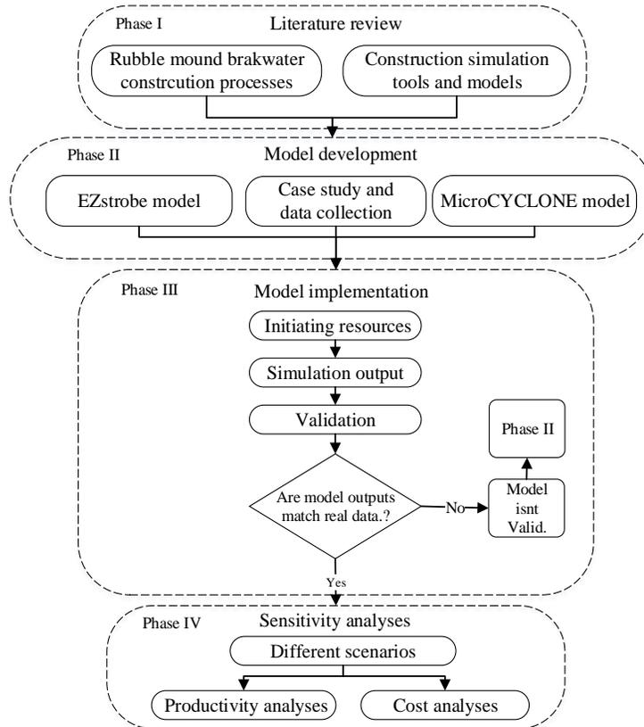
Figure 2: Simulation methodology of rubble-mound breakwater construction
