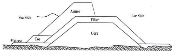
Figure1: Rubble-mound breakwater typical section
