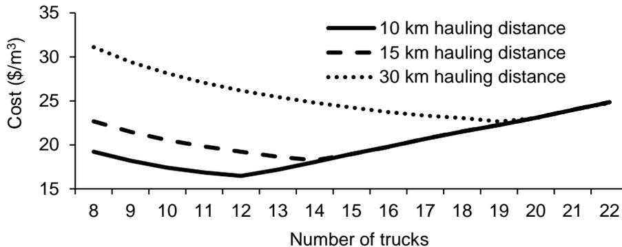
Figure 8: Average cost using 2 loaders and 3 placement backhoes
