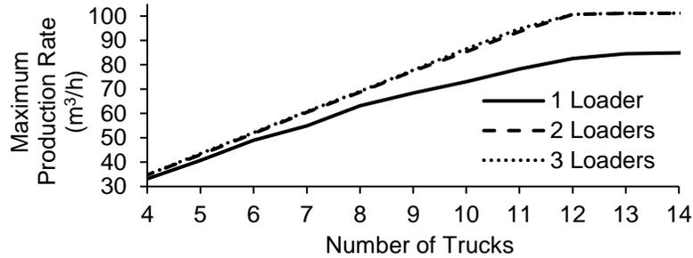
Figure 5: Max. production rate for different scenarios of 10 km hauling distance
