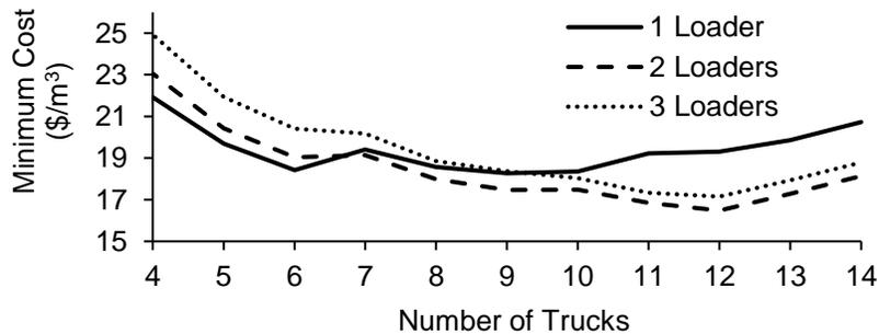
Figure 6: Minimum average cost for different scenarios of 10 km hauling distance
