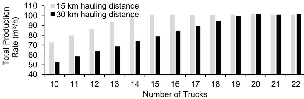
Figure 7: Total production rate using 2 loaders and 3 placement backhoes
