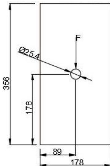
Figure 1: Parallel to the grain specimen (dimensions in mm)
