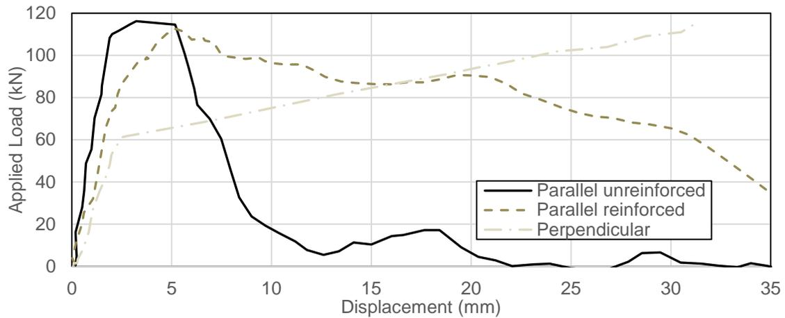
Figure 14: Typical load-deformation curves for dynamic tests
