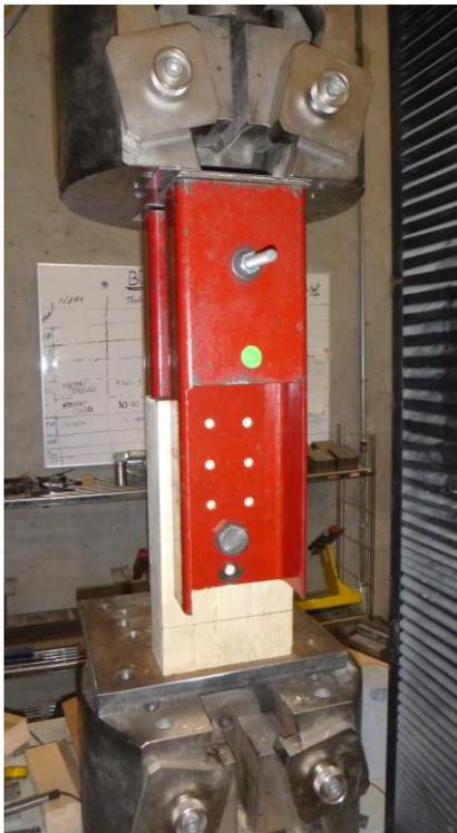
Figure 5: Parallel to the grain static test
