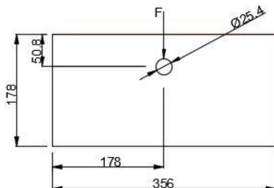
Figure 2: Perpendicular to the grain specimen (dimensions in mm)
