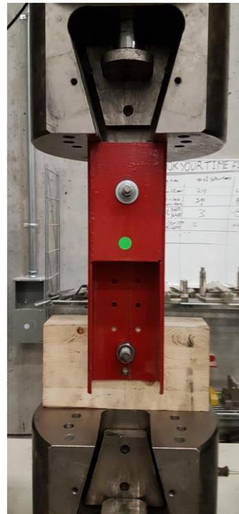
Figure 6: Perpendicular to the grain static test
