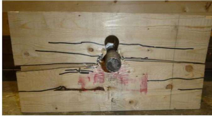
Figure 13: Specimen E90D[2] after dynamic test
