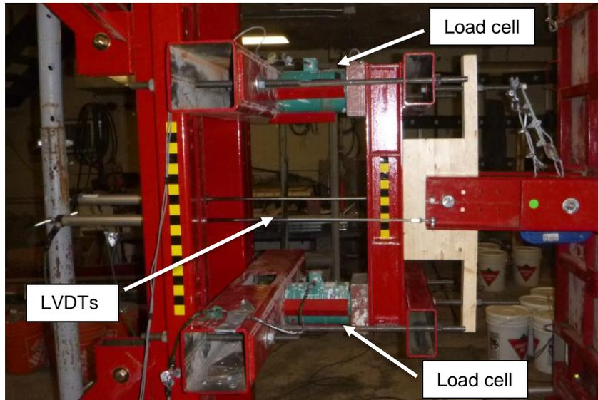
Figure 8: Instrumentation for dynamic tests
