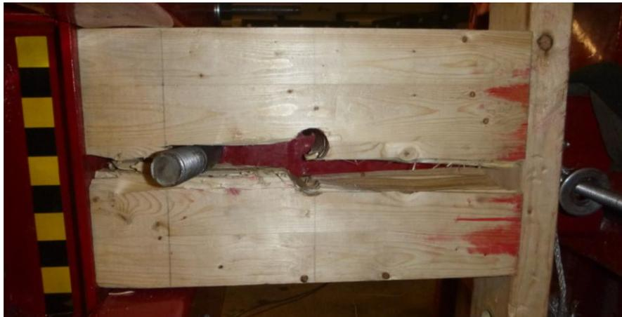
Figure 11: Splitting of specimen E0D[3]
