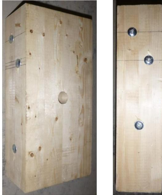
Figure 4: Screw reinforcement detail
