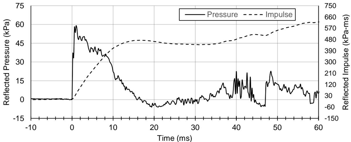
Figure 10: Typical reflected pressure and impulse time history
