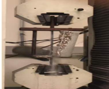
Figure 5: Carbon FRP Reinforced Cylinder
