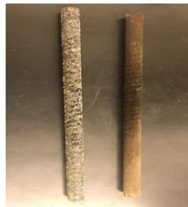
Figure 3: Basalt FRP before (left) and after (right) heating
