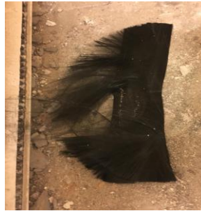
Figure 2: Carbon FRP bars after 2 hours at 600°C
