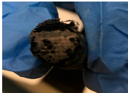
Figure 1: Surface degradation of steel specimen
