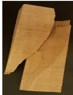
Figure 10: Failure of sample at elevated temperature
