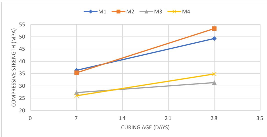
**Fig 2: Compressive Strengths of Test Cubes**
