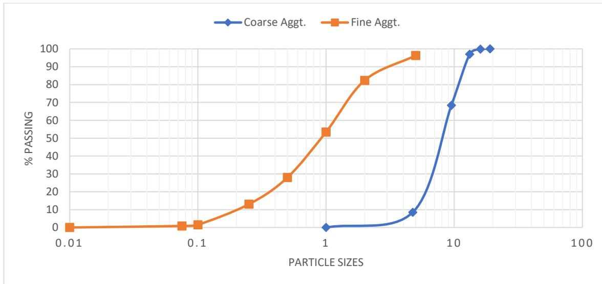
**Fig 1: Sieve Analysis of the Fine and Coarse Aggregate**
