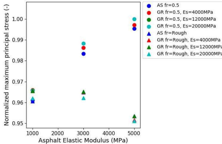
Figure 6: Maximum stresses in loaded panel for nighttime temperature gradient
