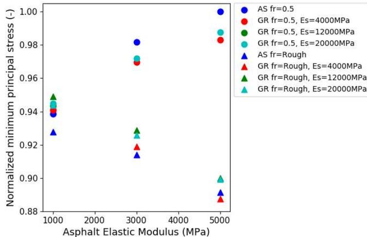
Figure 7: Minimum stresses in loaded panel for nighttime temperature gradient
