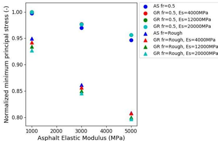
Figure 5: Minimum stresses in loaded panel for daytime temperature gradient
