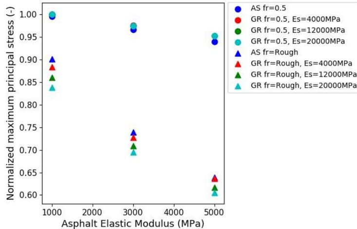
Figure 4: Maximum stresses in loaded panel for daytime temperature gradient
