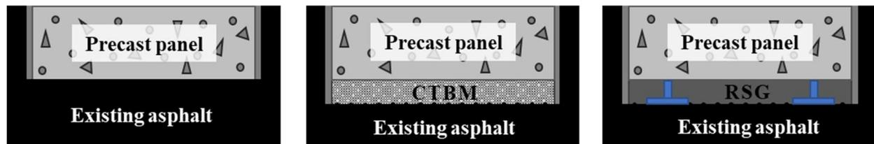
Figure 2: Support condition alternatives (L to R: asphalt-supported, grade-supported, and grout-supported)
