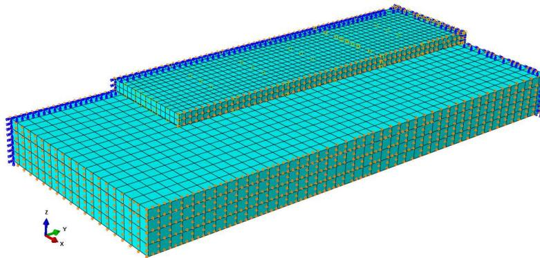
Figure 3: Finite element model of precast concrete inlay panels
