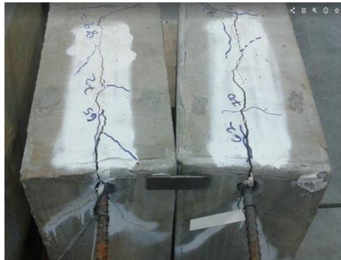
Figure 3 Splitting failures of tested specimens
