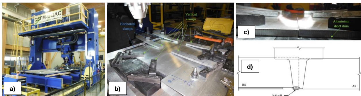
Figure 3: FSW setup a) Gantry b) Clamping system c) Aluminium sheet shim under AS d) Aluminium sheet shim under RS details
