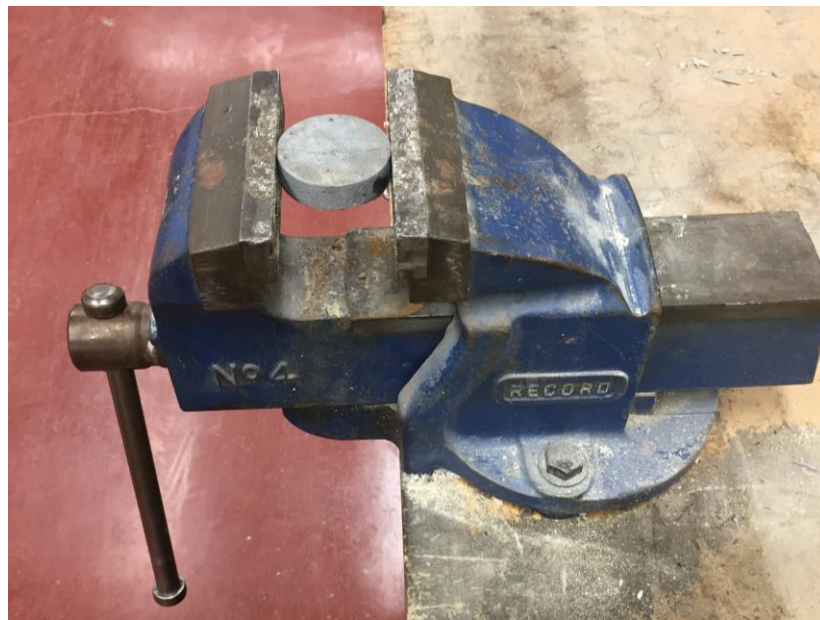
Figure 1: Cracking of specimens using screw jack
