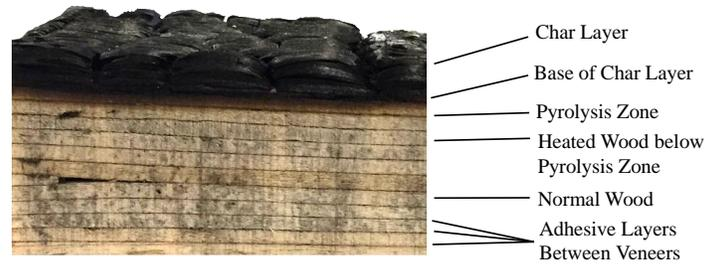
Figure 1: Timber breakdown when heated (Laminated Veneer Lumber shown)
