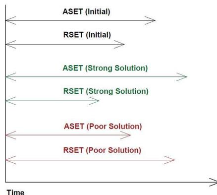
Figure 3: Possible ASET and RSET outcomes for strong and poor engineering solutions (taking both structural, behaviour and disability into account)
