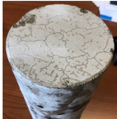
Figure 4: Core sample taken from the box unit from Meatbird Creek Culvert in wet state
