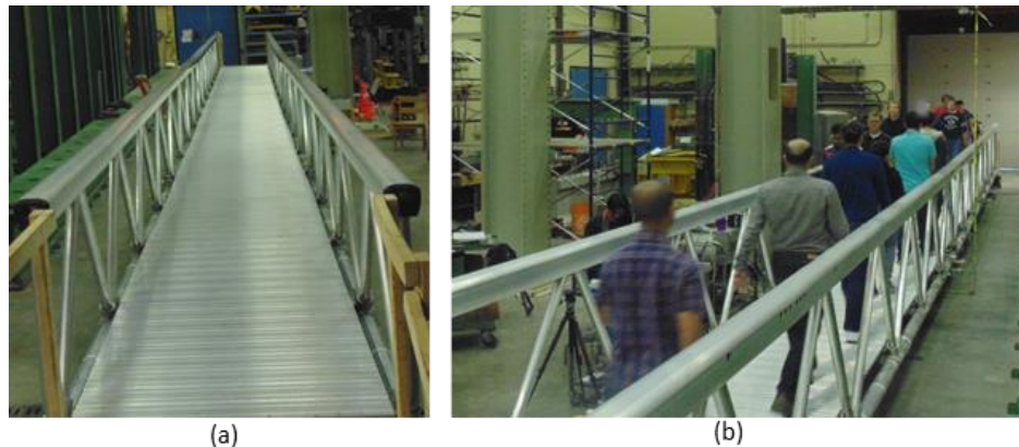
Figure 1: (a) 22.9 m bridge specimen, and (b) crowd tests on the bridge
