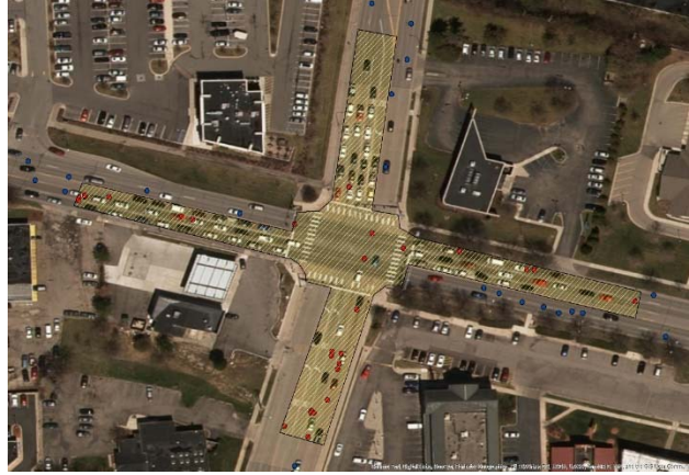
Figure 1: Intersection influence area (shaded in yellow) and an example of the candidate intersection events (red dots) and segment events (blue dots).
