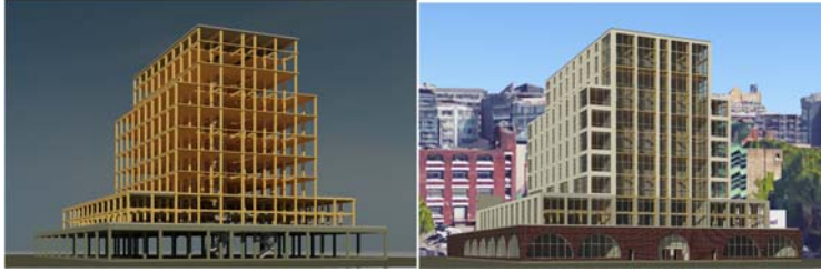
Figure 1: Structure of Hypothetical A engineered timber hybrid building (left), and exterior of Hypothetical A building (right).
