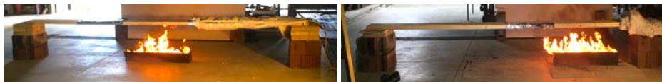
Figure 3: Test setup of the heating portion of the experiment for the moment region (left) and the shear region (right), in which the 4.2m Glulam beams were exposed to a pool fire for approximately 5 minutes on each side
