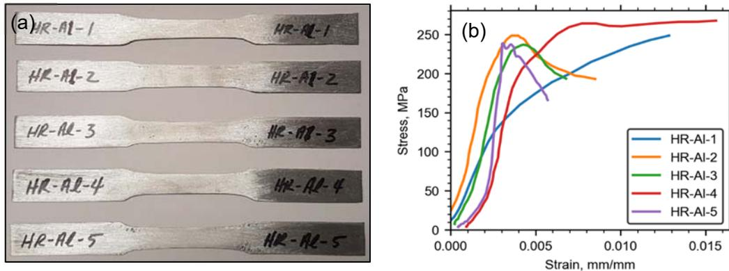
Figure 2: Test method verification (a) specimens (b) stress-strain results of HR-AI test specimens
