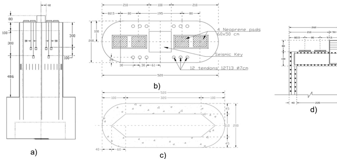
Figure 1. Typical pier details: a) Elevation view, b) Top view, c) Hollow section, d) Solid Section (Note: dimensions in cm) (MOPT, 2013)
