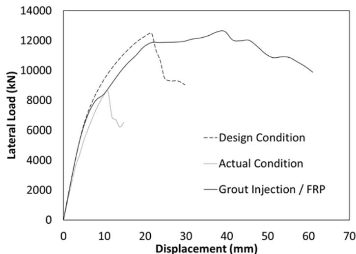
Figure 10. Comparison of capacity curves of the pier
