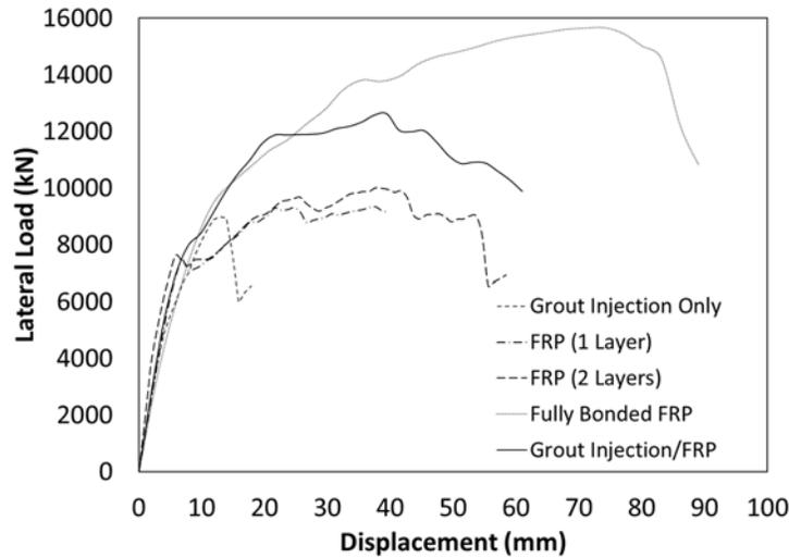
Figure 8. Rehabilitated pier capacity curves
