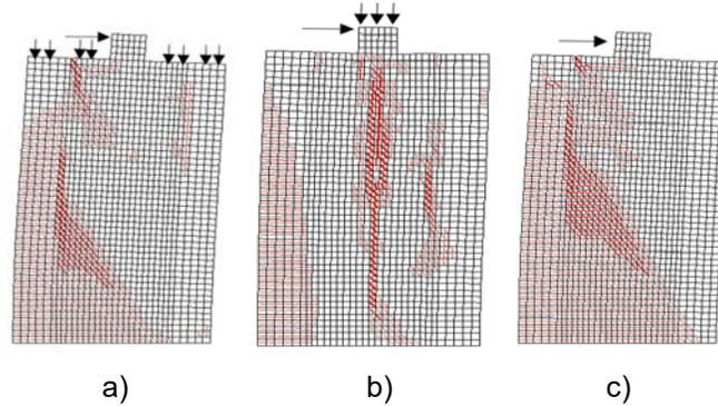
Figure 6. Cracking pattern and deformation at the peak load for: a) Design condition, b) Actual condition, c) Lateral load only.
