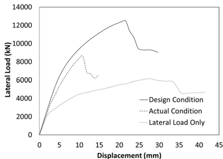
Figure 5. Bridge pier capacity curves.
