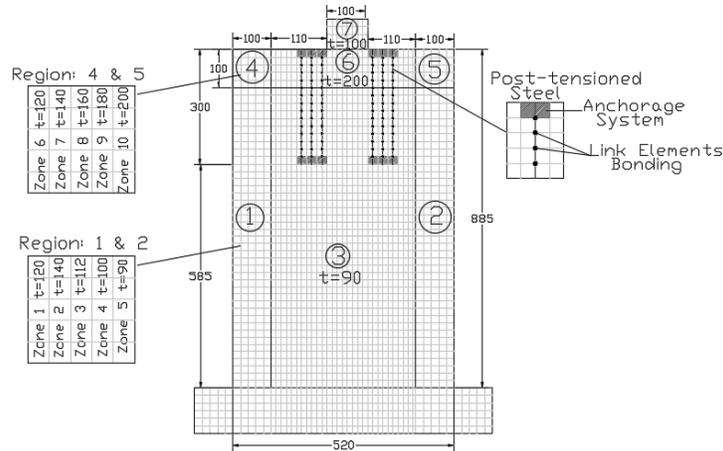
Figure 3. Finite element model of the pre-rehabilitated pier
