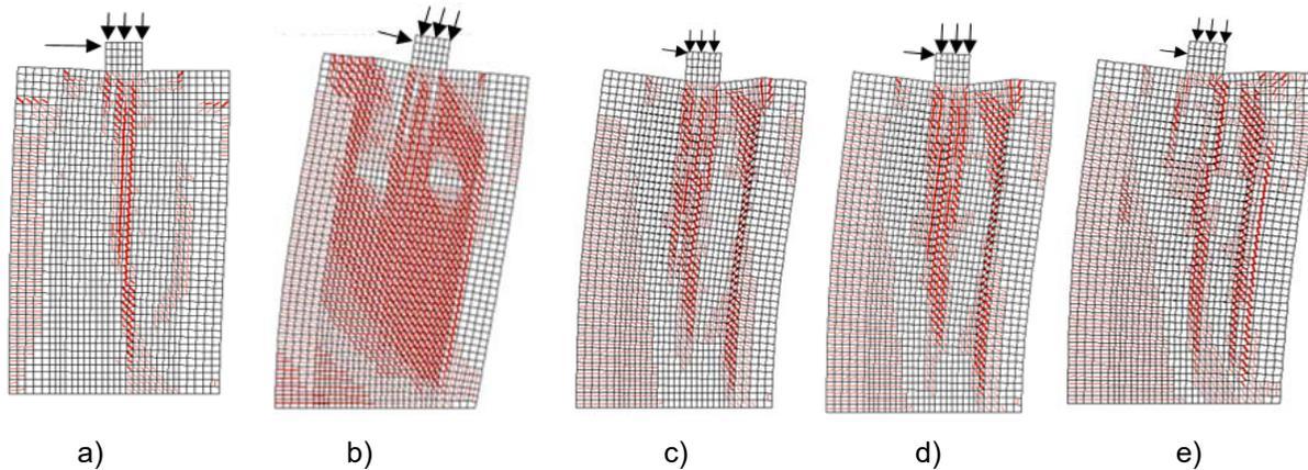
Figure 9. Cracking pattern and deformation at the peak load for rehabilitated pier with: a) Grout injection, b) Fully bonded FRP, c) FRP (1 layer), d) FRP (2 layers), e) FRP with Grout injection
