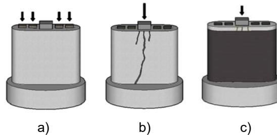
Figure 2. States of the structure: a) Design condition, b) Actual condition, c) Rehabilitated condition
