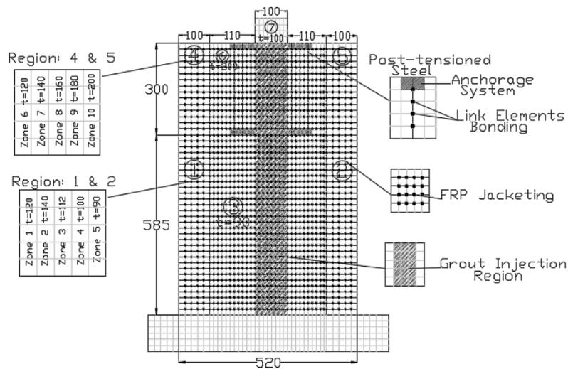
Figure 7. Finite element model of the rehabilitated pier
