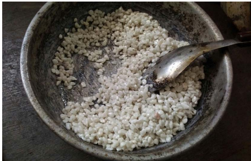
Figure 4: UP resin mixture blended with alabaster
