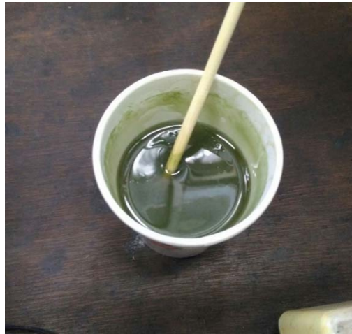
Figure 3: UP resin mixed with accelerator and hardener
