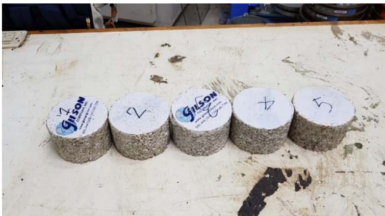
Figure 2: The 4-in specimens of compacted UP mixtures
