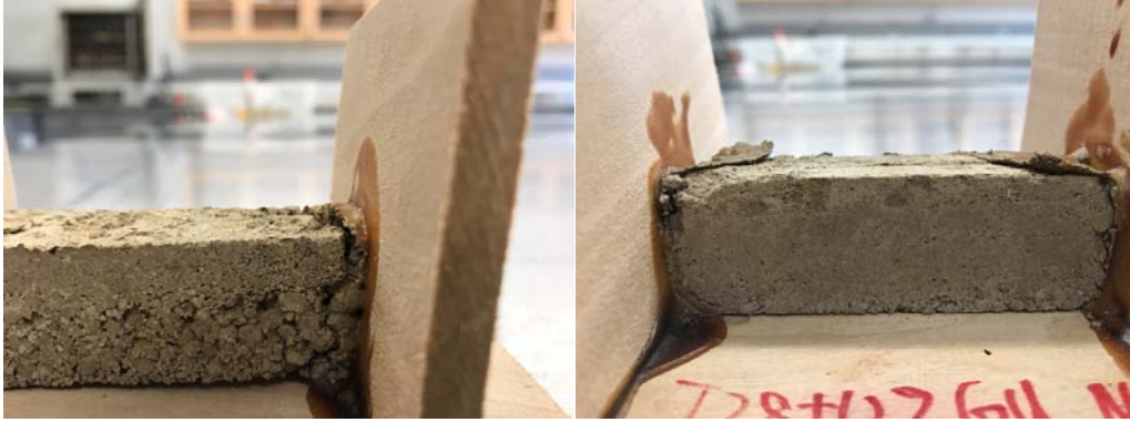
Figure 6: State of soil beams Blenheim clay with 12% GU NM after 3 cycles (left), Dresden silt with 12% GU NM after 10 cycles (right)
