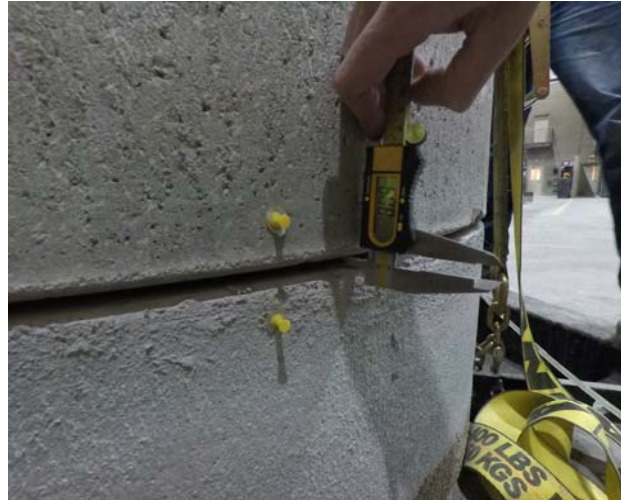
Figure 8 Joint Gap Measurement During the Test
