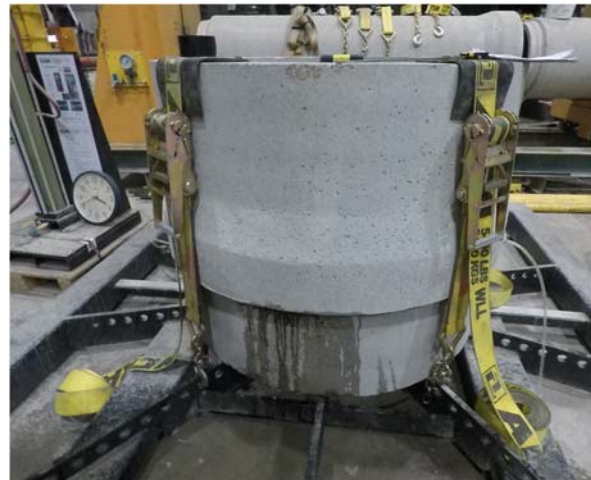
Figure 10. 900 mm RCP Test at 600 kPa
