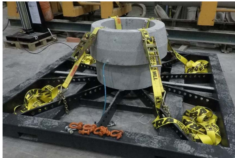
Figure 4 Base frame and test pipe setup
