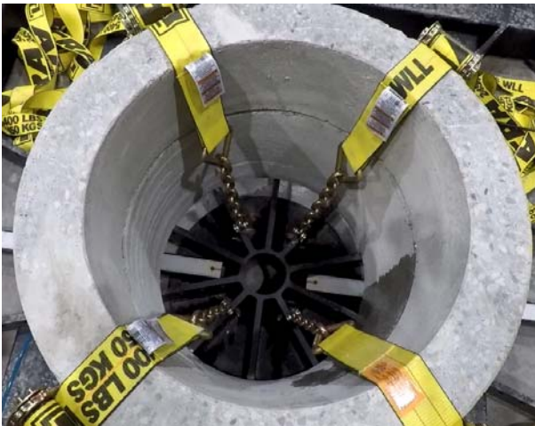
Figure 9. 600mm RCP with T02 at 250 kPa
