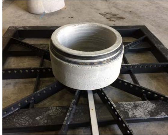
Figure 6 Testing and secondary gasket setup
