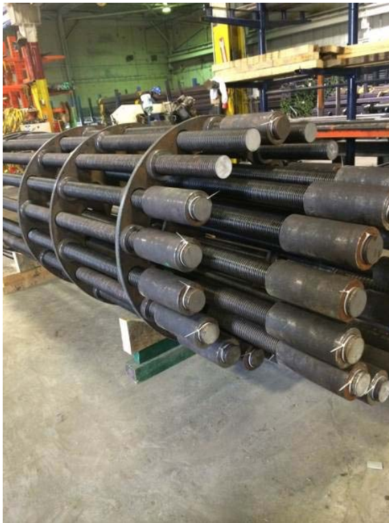
Fig. 10: a) Multi-ring Caisson splice concept
