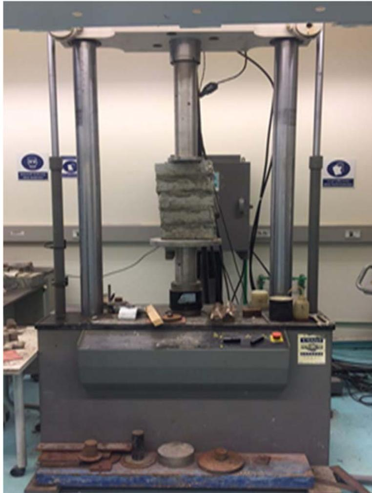
Figure 1: A prism sample during testing it under compression.
