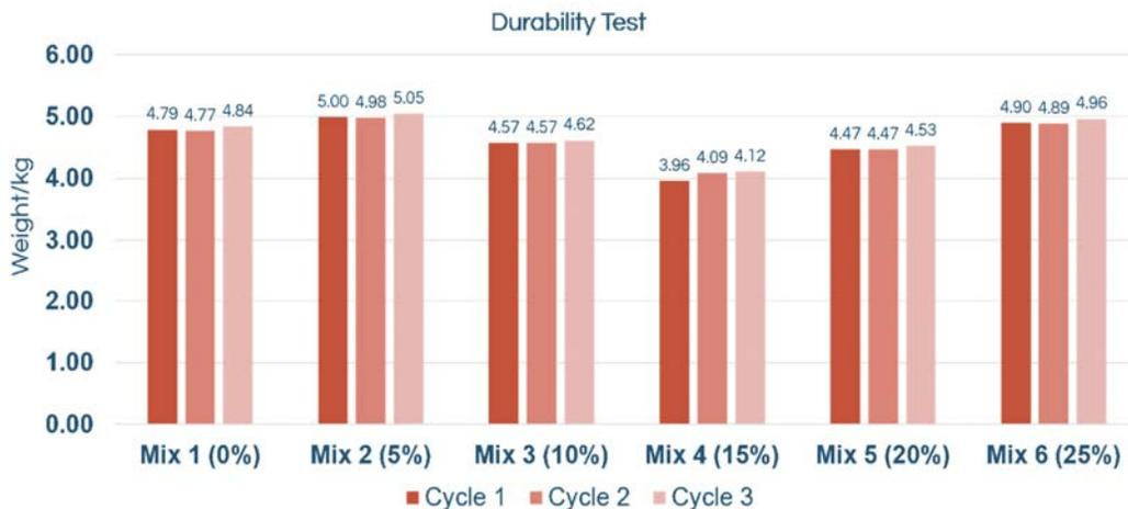
Figure 3: Cycles of immersion in salt solution
