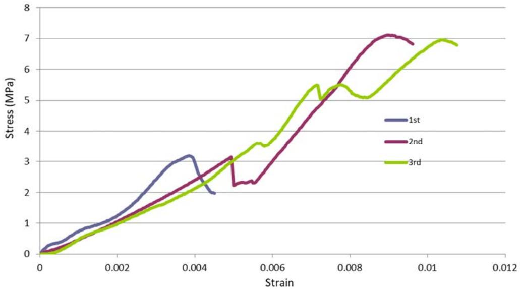
c. Stress-strain curve for the 10% slurry prism sample.
