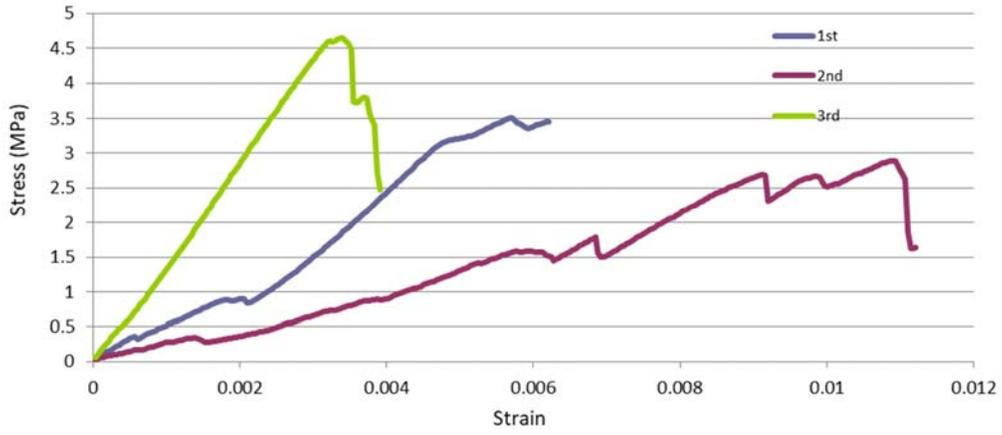
a. Stress-strain curve for the 0% (control) prism sample.
