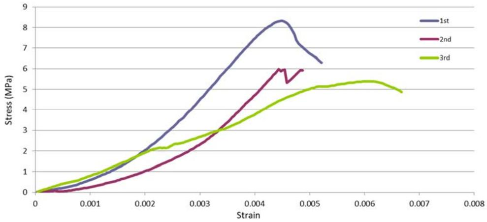
b. Stress-strain curve for the 5% slurry prism sample.
