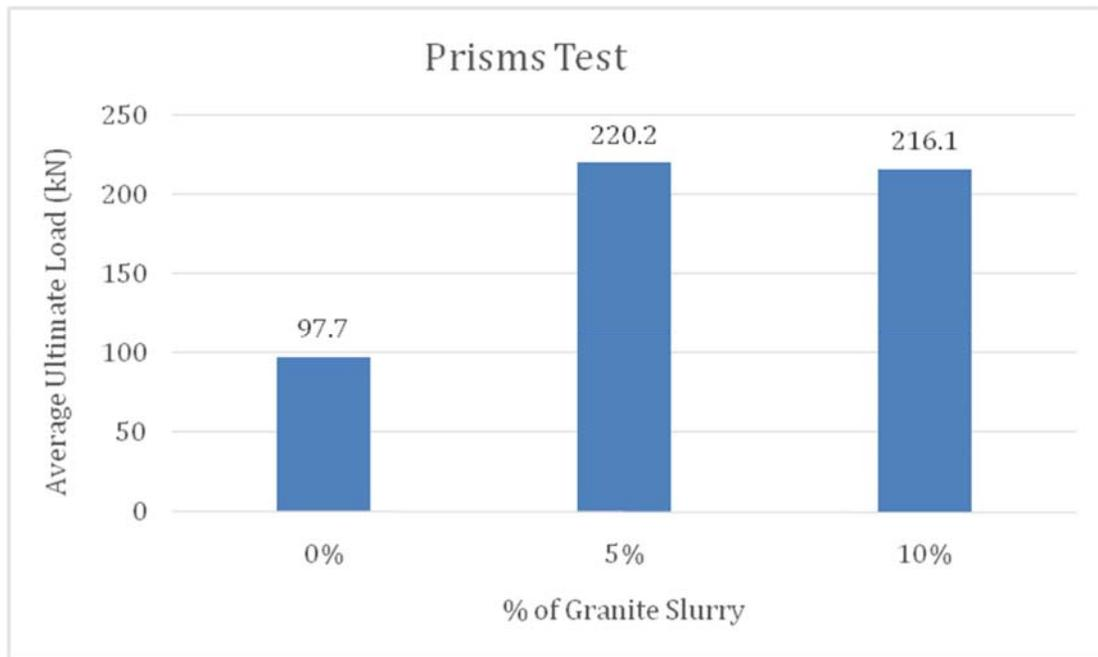
Figure 1: The average ultimate load carried by prisms with different percentages of slurry.
