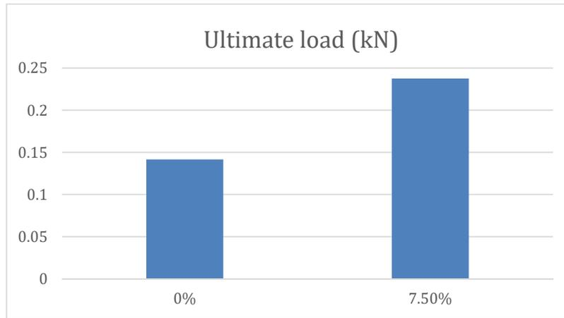
Figure 2: Comparison between the ultimate compressive load carried by the control mortar sample and the mortar sample containing 7.5% slurry
