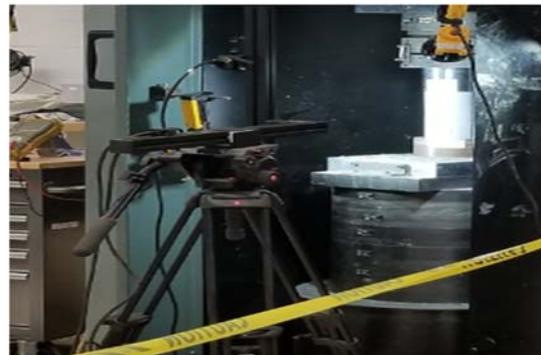
Figure 3: DIC setup
