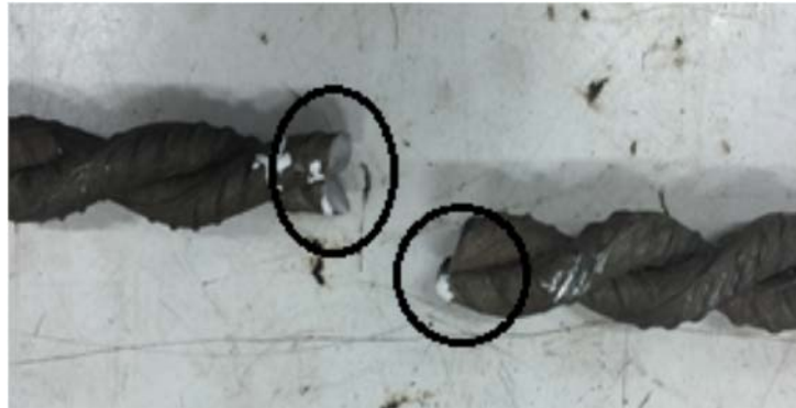
Figure 10: The mode of failure of the spun steel specimen.
