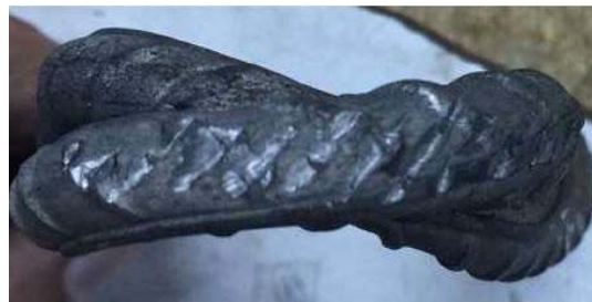
Figure 11: Side view of the cold-bent specimen
