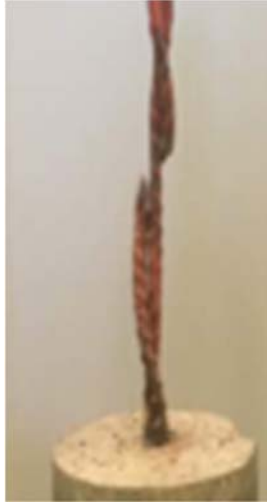
Figure 7: The Failure mode of spinned steel specimen
