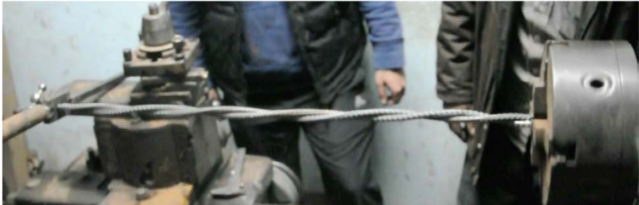
Figure 1: Twisting the bars using the power lathe
