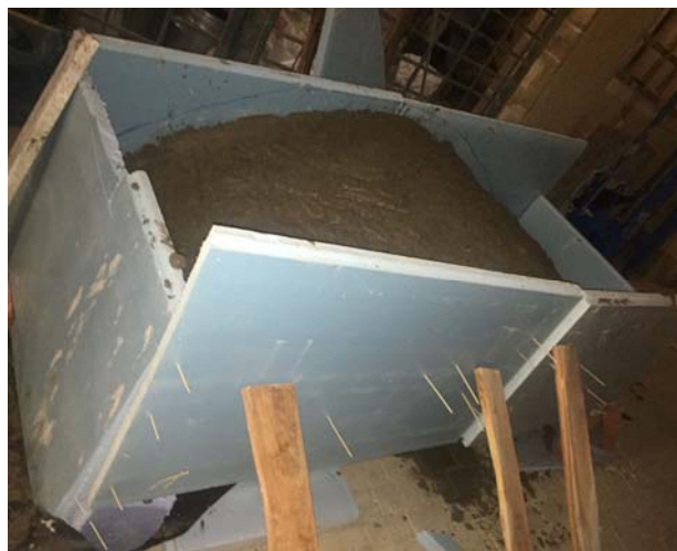
Figure 9: Curved Sample After Pouring
