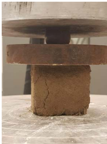
Figure 3: Compressive Failure of Selected Batch
