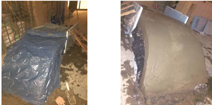
Figure 10: Curved Sample During Curing
