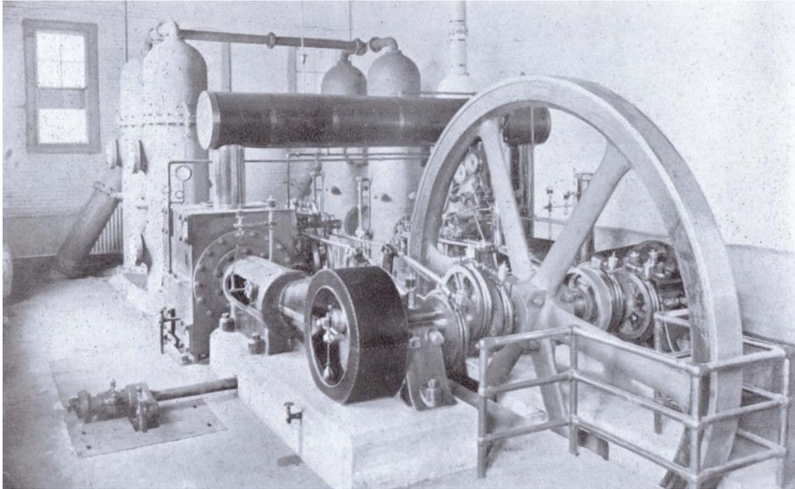
Figure 6. Allis-Chalmers compound Corliss pumping steam engine at the Fredericton Pumping Station and Water Treatment Plant (c. 1906). Installed in 1906 and removed in 1955. [Source: Provincial Archives of New Brunswick Image: P657-28]
