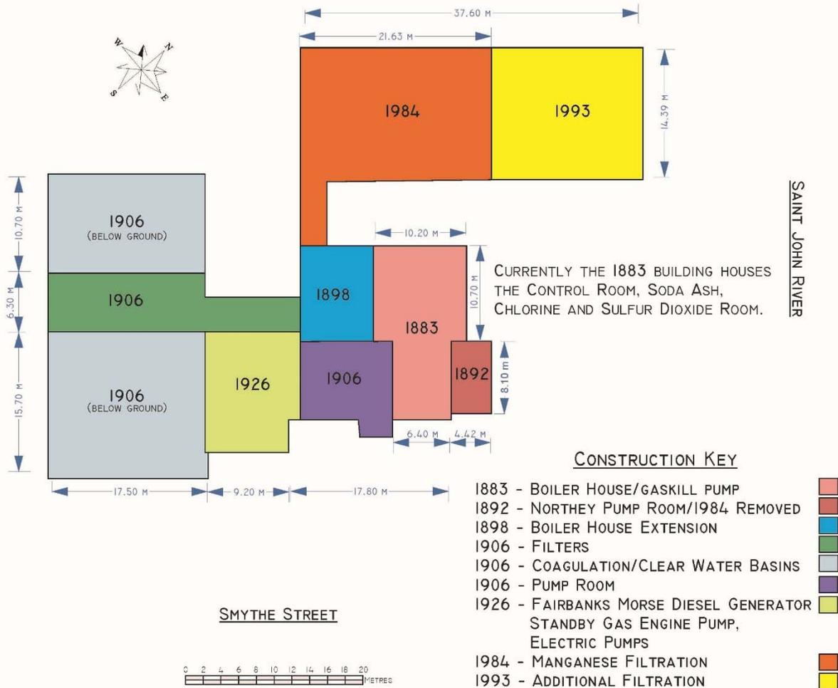
Figure 1: Footprint of the 1883 water treatment plant and extensions between 1883 and 1993
