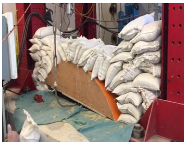
Figure 1: Arched sandbags system
