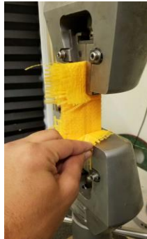
Figure 3: Tensile test on the sandbags polypropylene material
