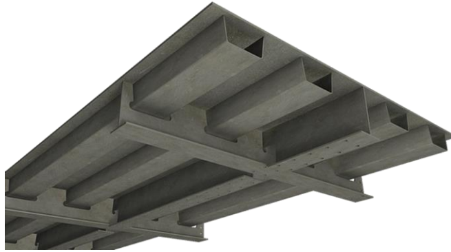
Figure 1: Typical orthotropic steel deck section
