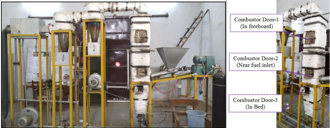
Figure 3: Actual picture of Bubbling Fluidized Bed Unit
