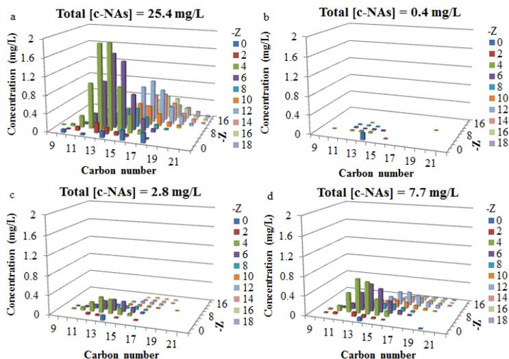
**Figure 1.** NA distribution in a) raw OSPW, and OSPW treated with b) UV-NTA-Fenton, c) UV- $\text{H}_2\text{O}_2$ , and d) NTA-Fenton ( $[\text{H}_2\text{O}_2]_0 = 5.88$  mM for all three processes.  $[\text{Fe}]_0 = 0.089$  mM and  $[\text{NTA}]_0 = 0.72$  mM for UV-NTA-Fenton and NTA-Fenton. 30 min UV irradiation for UV-NTA-Fenton and UV- $\text{H}_2\text{O}_2$ ) (Zhang et al., 2016).
