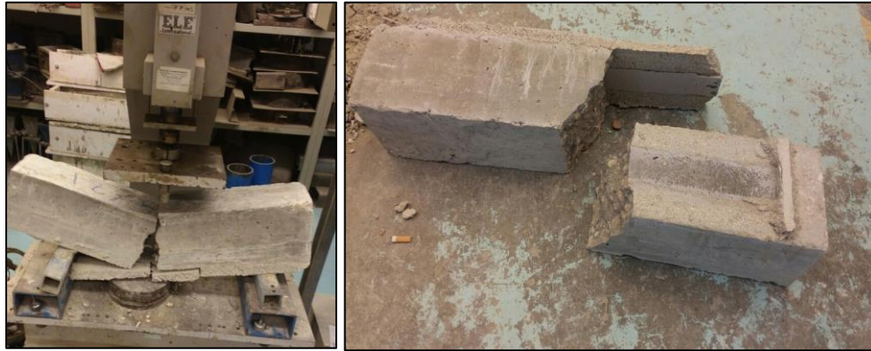
Figure 9: Typical failure mode for the CFRP protected beams
