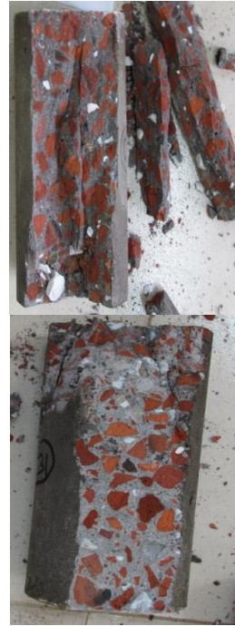
Figure 6 Concrete failure by compression (PAC10-W42 & PAC10-W57).
