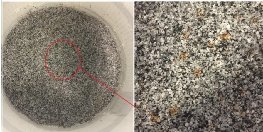
Figure 4. Rust in aggregate crushed in the disk pulveriser with iron plates.
