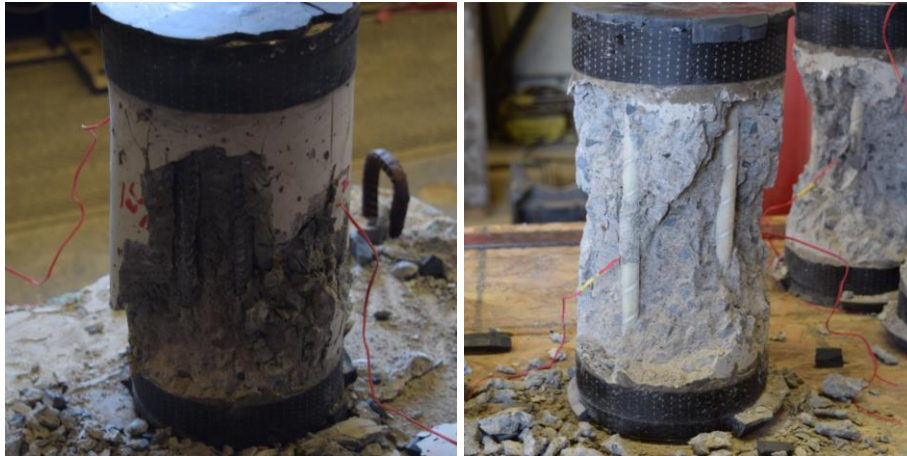
Figure 2: Typical failure mode of specimens reinforced with steel (left) and GFRP (right) bars
