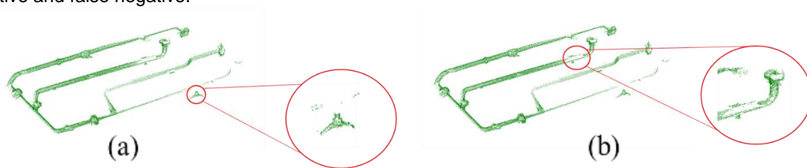
Figure 5. Challenges of removing clutter points without removing points on the object of interest. (a) Example of remaining clutter points after clutter removal for K equal to 8. (b) Example of removed points from the object of interest for the same K value.
