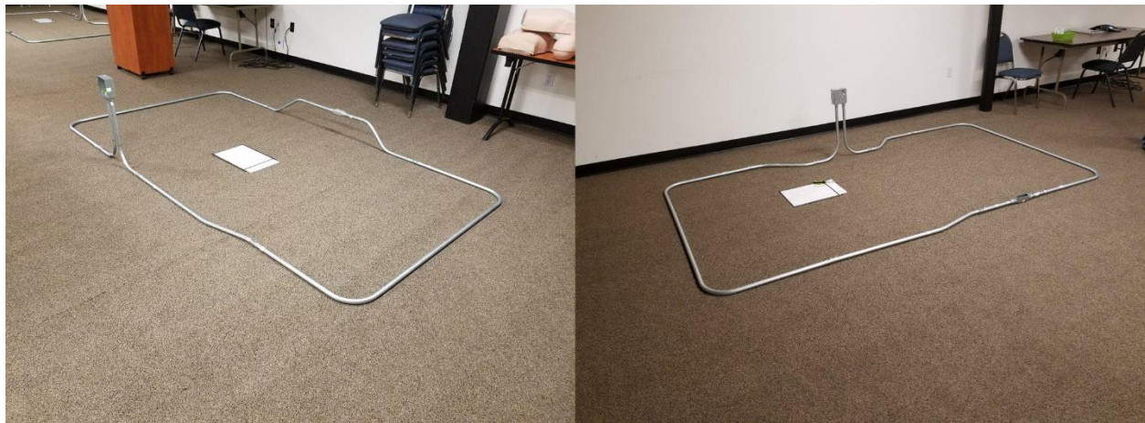
Figure 1: The two conduit assemblies used
