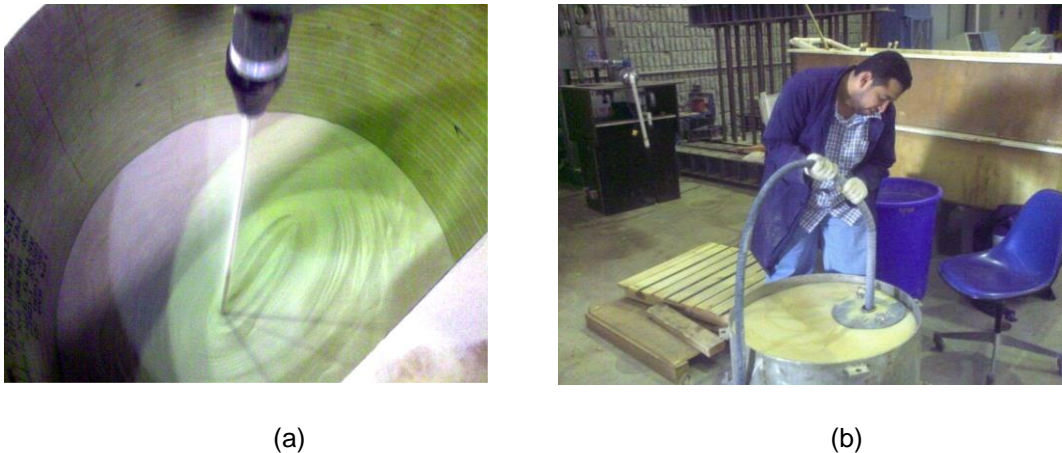
Figure 3: Densification and density control, (a) Pluviation technique, (b) Vibration technique.
