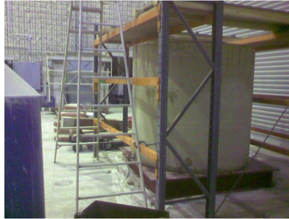
Figure 4: Soil chamber in the laboratory.
