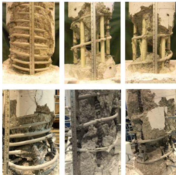
Figure 5: Columns after testing (in clockwise direction, starting from top left): P28-C-12-50, P28-C-12-160, P42-C-12-160, P28-LS-12-160, P41-LS-12-160, and P28-LS-12-50
