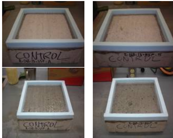
Figure 7 - Control mix at 0 cycles (top) and 50 cycles (bottom)
