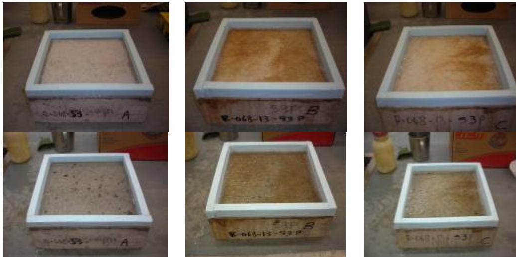
Figure 8 - 30% coarse RCA at 0 cycles (top) and 50 cycles (bottom)
