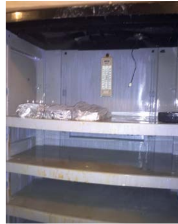
Fig.4b Bar Specimen in Moist Cabinet
