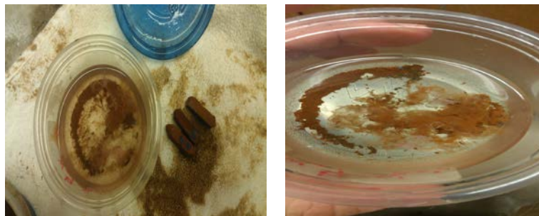
Figure 2: The MW oxidized samples and some iron oxidized precipitated in container
