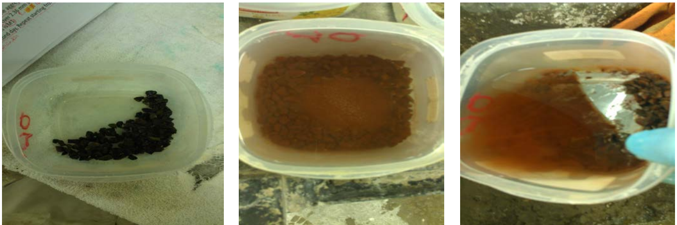
Figure 3: Progression of damage in Ore: left image: before testing, middle: after testing, and right: precipitation of iron hydroxides.
