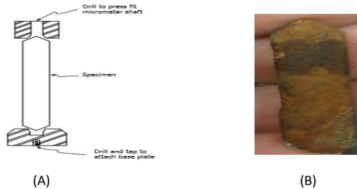
Figure 1: (A) The standard shape and size, adopted from ASTM C586 (B) Rock cylinder sample prepared in the lab
