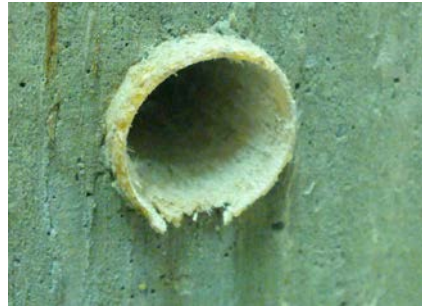
Figure 11 Residue of coating layer after pull-out
