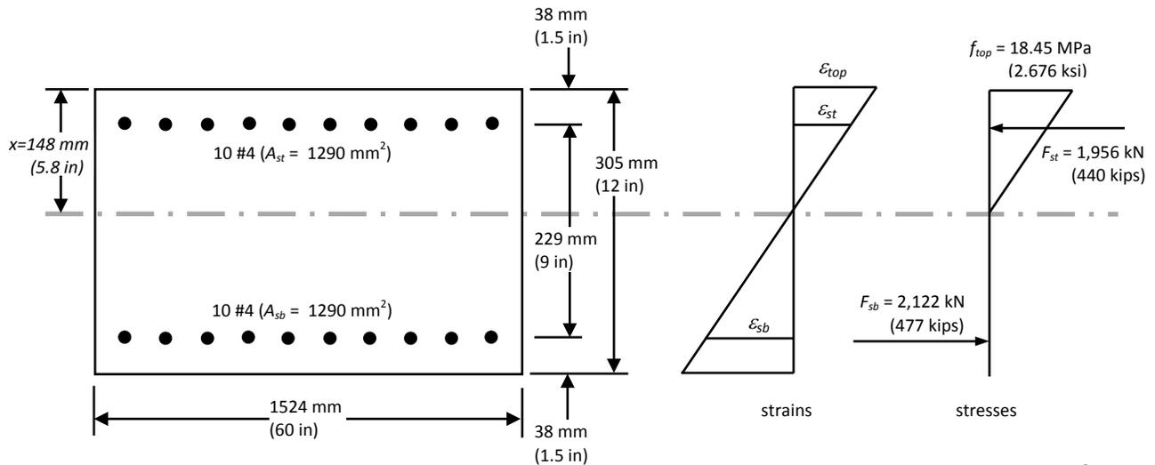
Figure 2: Flexural cross sectional analysis on RC segments reinforced with 20#4 bars ( $A_{\#4} = 129 \text{ mm}^2$ )
