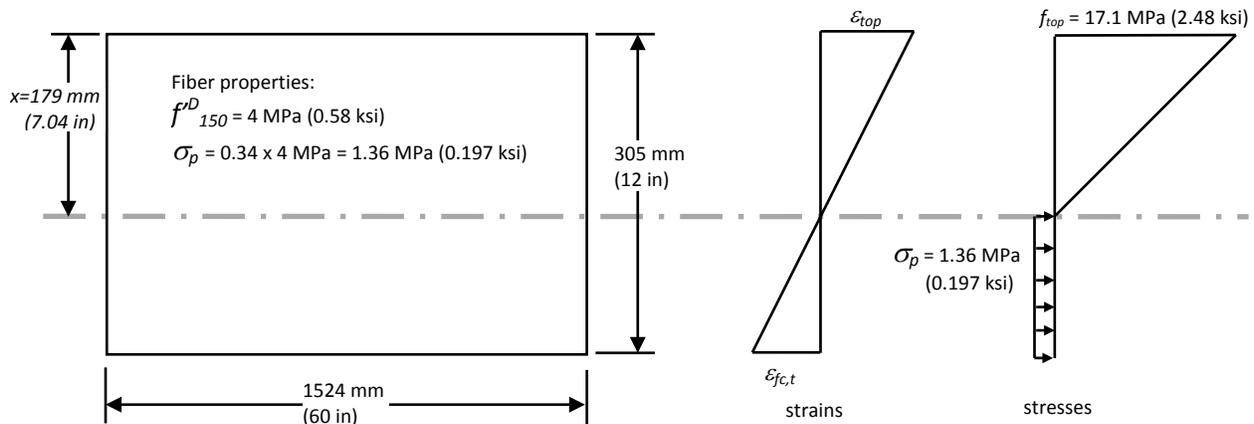
Figure 3: Flexural cross sectional analysis on FRC segments with ASTM residual parameter ( $f'_{D150}$ ) of 4 MPa (580 psi)
